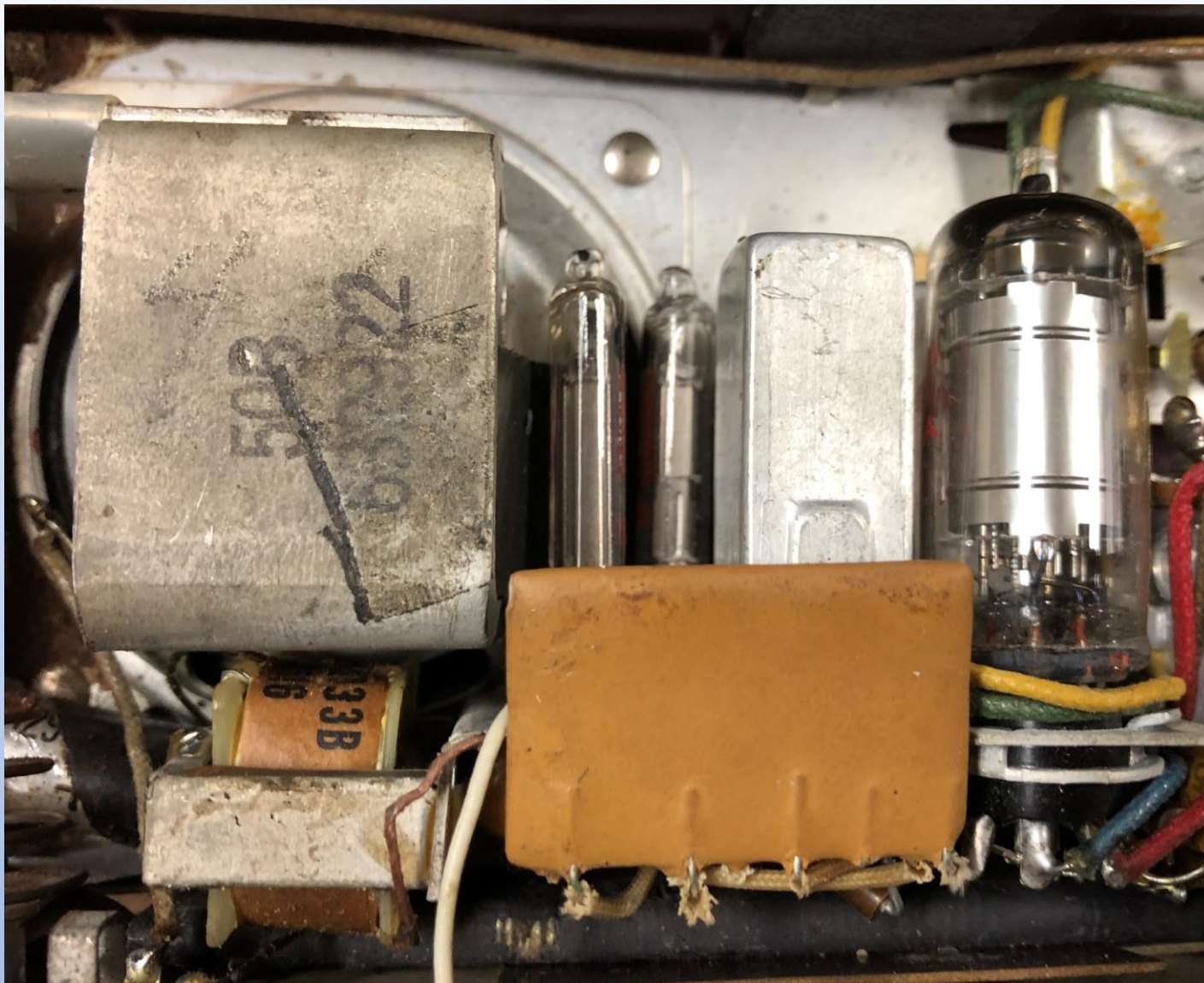
Interior of Motorola Pixie Radio – uses subminiature tubes created in World War II for military use
