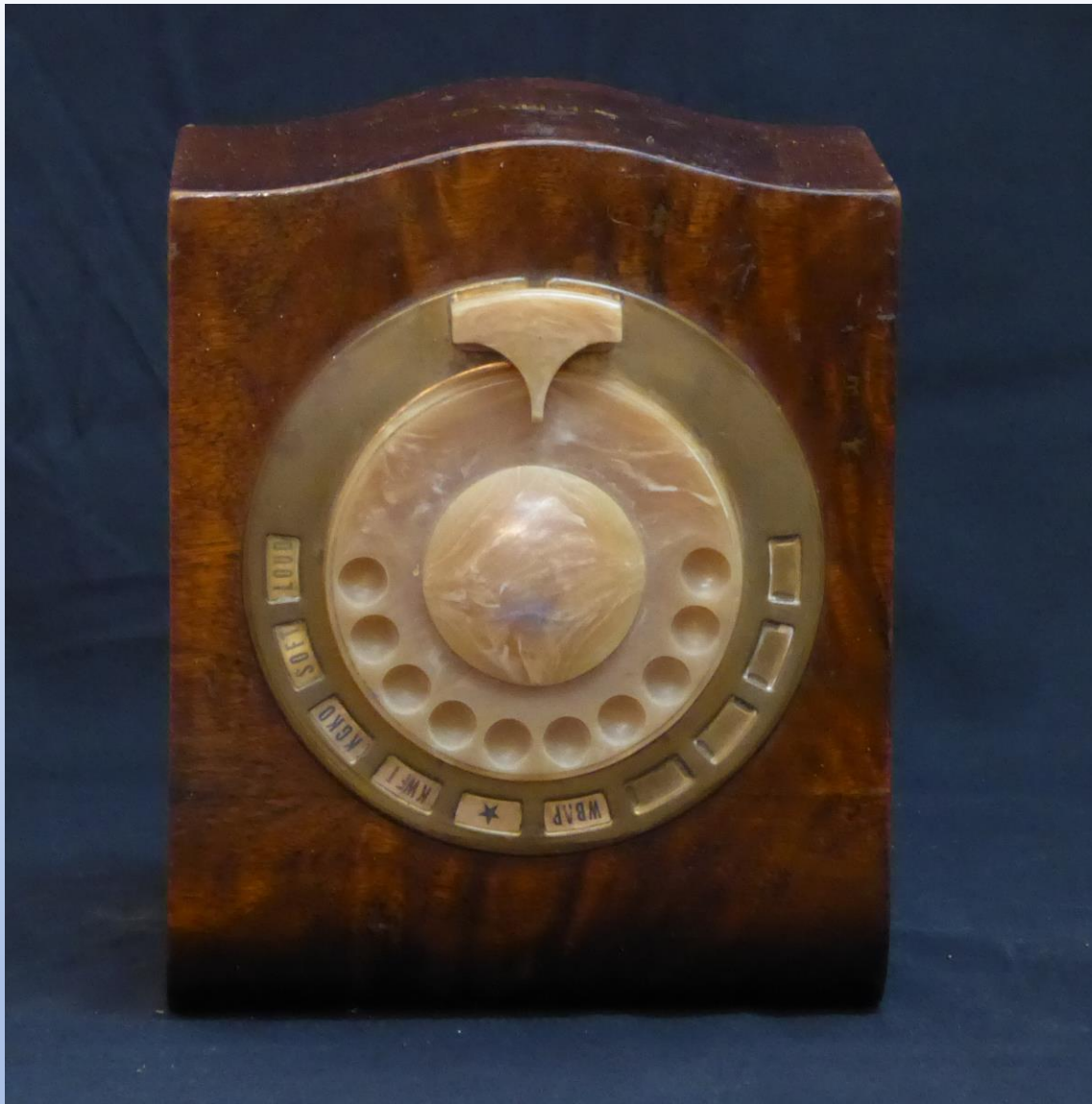
Philco 1939 "Mystery" Remote first home radio remote control not requiring any wires from remote to console
