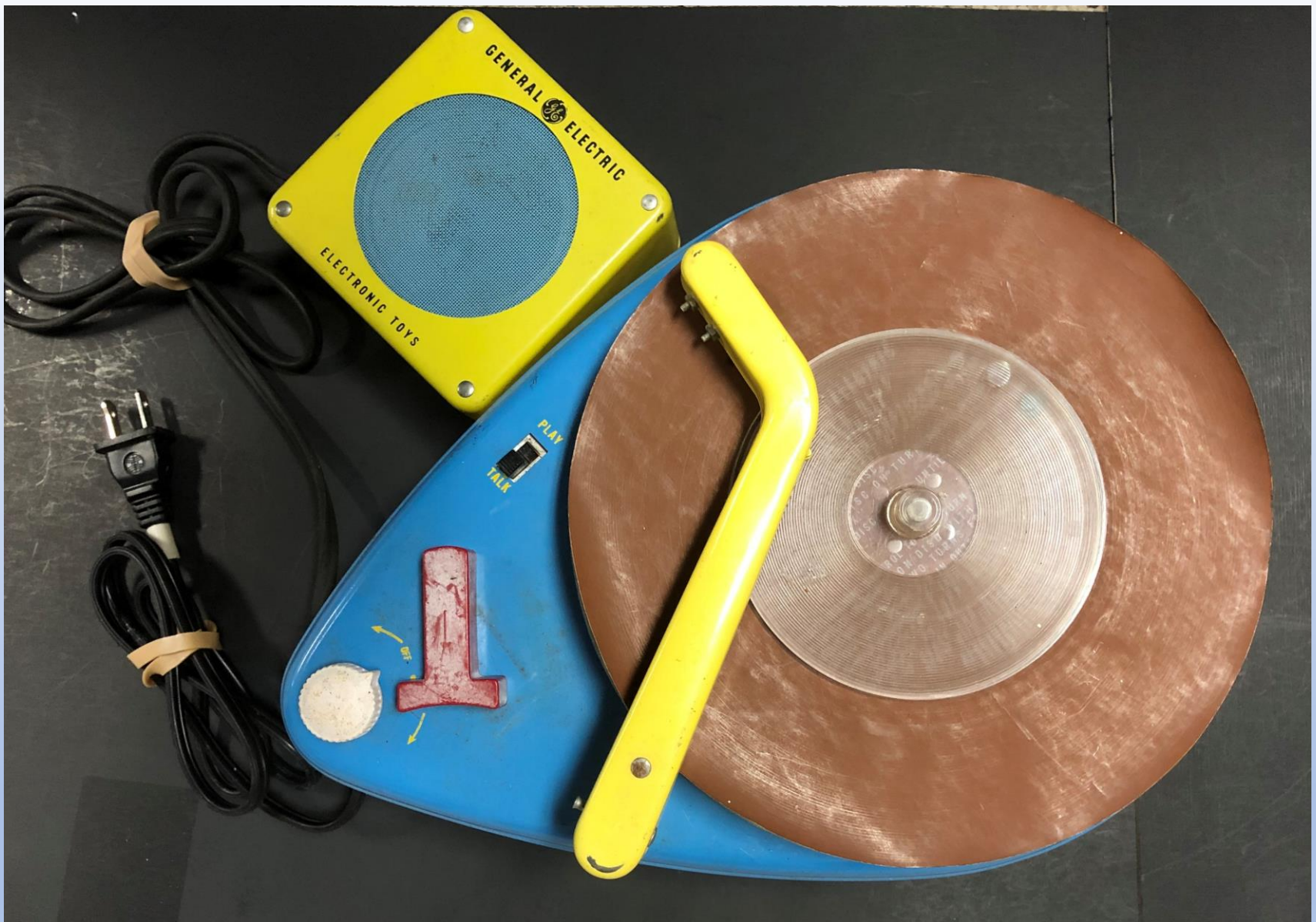
Late 1940s Child's Toy Recording Machine by General Electric (note the early "floppy disk" recoding media)
