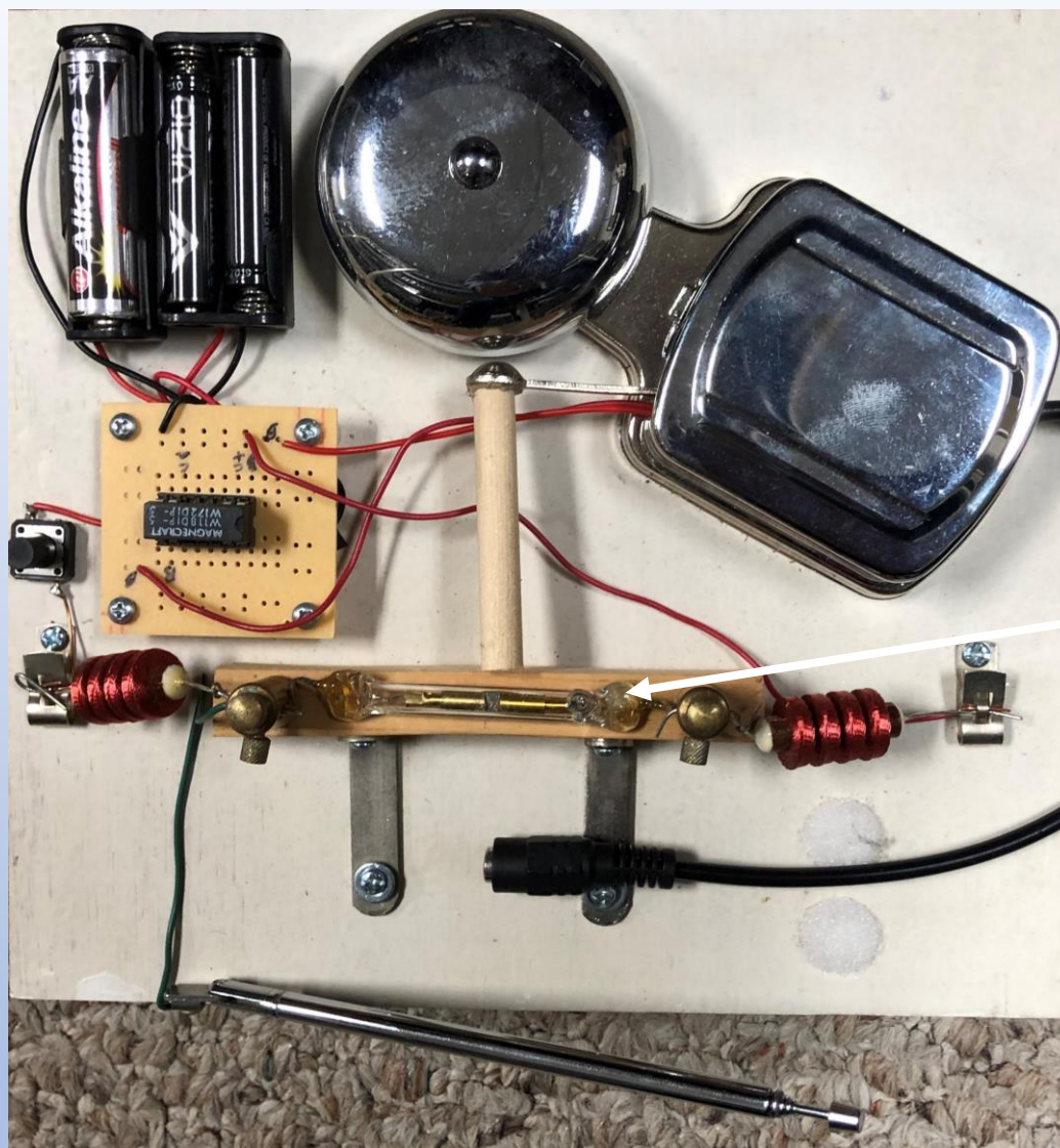
Modern Replica of Marconi's Early 1900s Coherer Receiver
