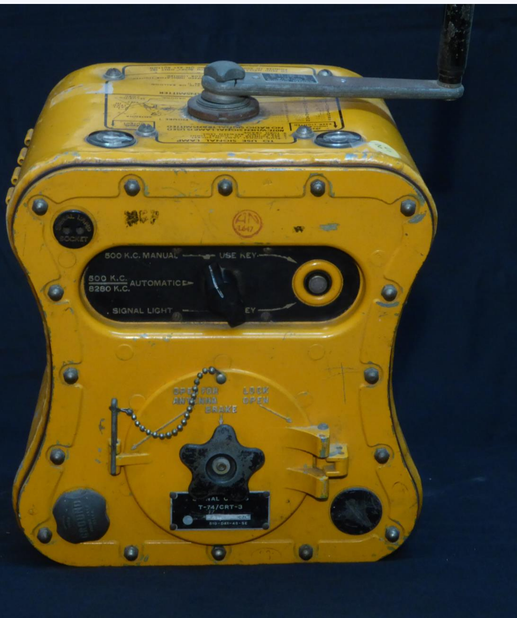
World War II “Gibson Girl” Life Raft Radio Turn the crank to send a homing signal to the rescue planes.
